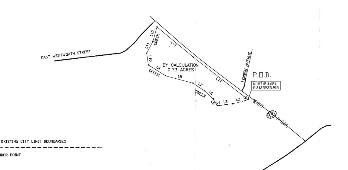
BEARING DISTANCE S 65'30'50" W 11.14 L2 S 75'54'30" W 44.90' L3 S 82'17'31" W 45.23' N 85'23'28" W 7.85 N 31°38'33" W 25.55 N 46'50'50" W 40.24 N 56'59'18" W 50.04 N 74'46'29" W 97.42 N 58'02'08" W 69.48 N 07'27'54" W 41.44
