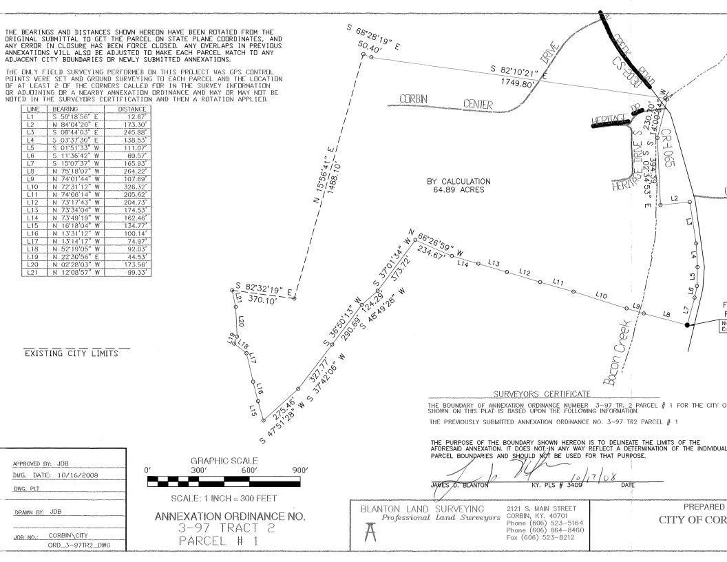
THE BEARINGS AND DISTANCES SHOWN HEREON HAVE BEEN ROTATED FROM THE ORIGINAL SUBMITTAL TO GET THE PARCEL ON STATE PLANE COORDINATES, AND ANY ERROR IN CLOSURE HAS BEEN FORCE CLOSED, ANY OVERLAPS IN PREVIOUS ANNEXATIONS WILL ALSO BE ADJUSTED TO MAKE EACH PARCEL MATCH TO ANY ADJACENT CITY BOUNDARIES OR NEWLY SUBMITTED ANNEXATIONS.
